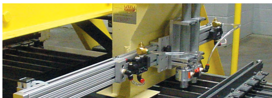
(2) Model 6083 1-1/2" (38mm) Line Vacs convey reject metal caps from a fluorescent lamp operation to a scrap bin.
