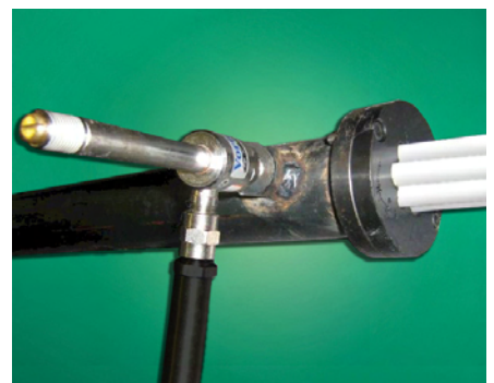
Cold air from a Model 3230 Vortex Tube quickly cools extruded plastic tubing.
