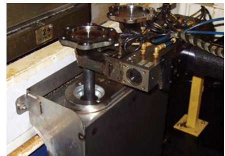
The flanged end of an axle is lifted through a Super Air Wipe to blow off chips after machining.
