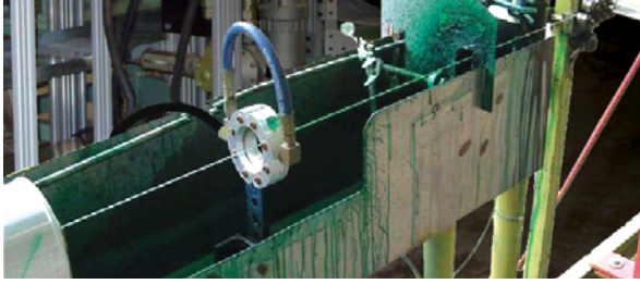
A Model 2431 1" (25mm) Standard Air Wipe blows off the excess coating from a wire into a dip tank.
