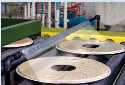
The 54" (1372mm) Super Air Knife dries stamped parts that exit a washer.
