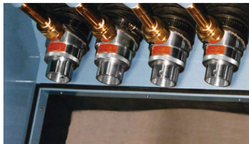
Adjustable Air Amplifiers are ducted to draw clean air for drying.
