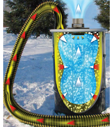
This special air amplifier is used to draw polluted air through an activated charcoal filter.
