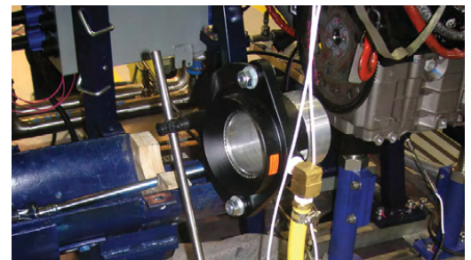
A Model 120024 4" (102mm) Super Air Amplifier cools an engine during dynamometer testing.
