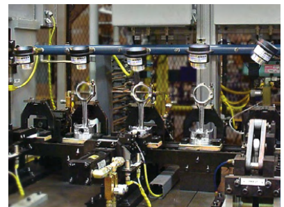
(5) Model 120022 2" (51mm) Super Air Amplifiers cool truck pistons prior to gauging.
