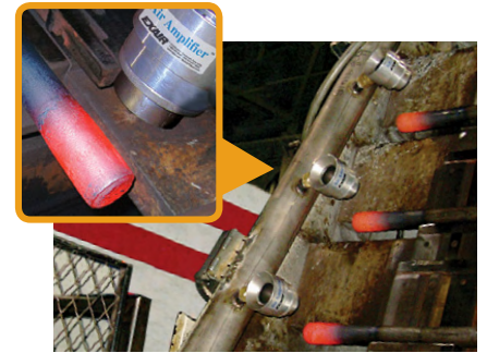
Model 6042 2" (51mm) Adjustable Air Amplifiers with swivel fittings cool inductively heated axles prior to installing the hubs.
