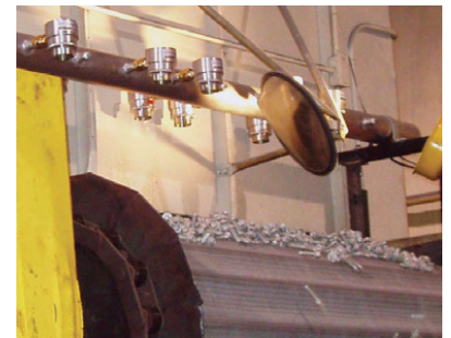
Metal parts are dried using a series of Model 6042 2" (51mm) Adjustable Air Amplifiers.
