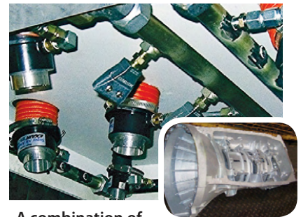
A combination of Model 120022 2" (51mm) Super Air Amplifiers and Model 1122 2" Super Air Nozzles blow off transmissions after they are machined.
